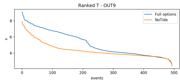
Figure 8 Maximum period for each TC event ranked. Orange are simulation without tide and blue with tide. at station OUT9 in the East Arm
