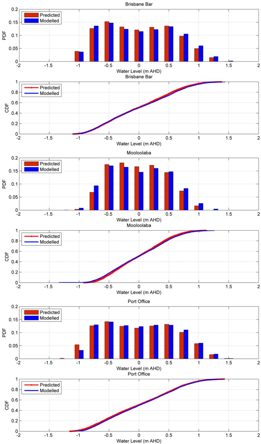
Figure 5-2 Statistical comparison of modelled and measured tide
