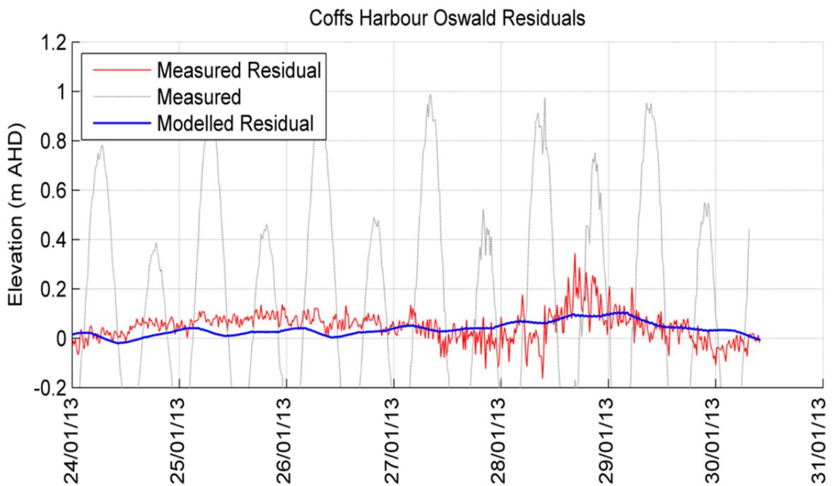
Figure 5-9 (contd.) Measured and initial RHM-modelled tidal residuals during Ex-TC *Oswald*
