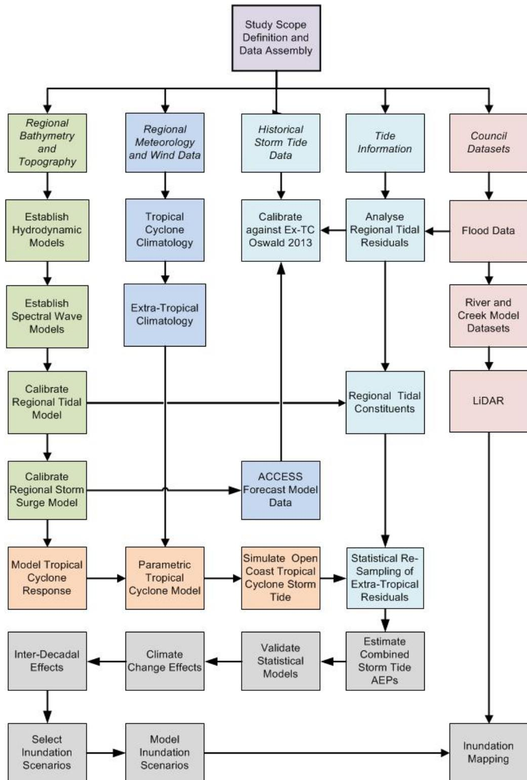
Figure 2-1 Overview of the Storm Tide Hazard Methodology
