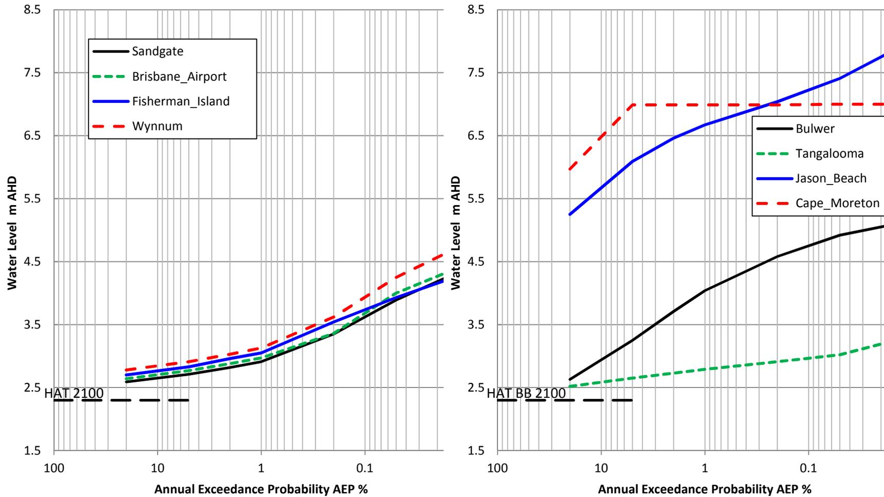
Figure 7-8 Combined 2100 climate breaking wave runup estimates at selected sites<sup>26</sup>
