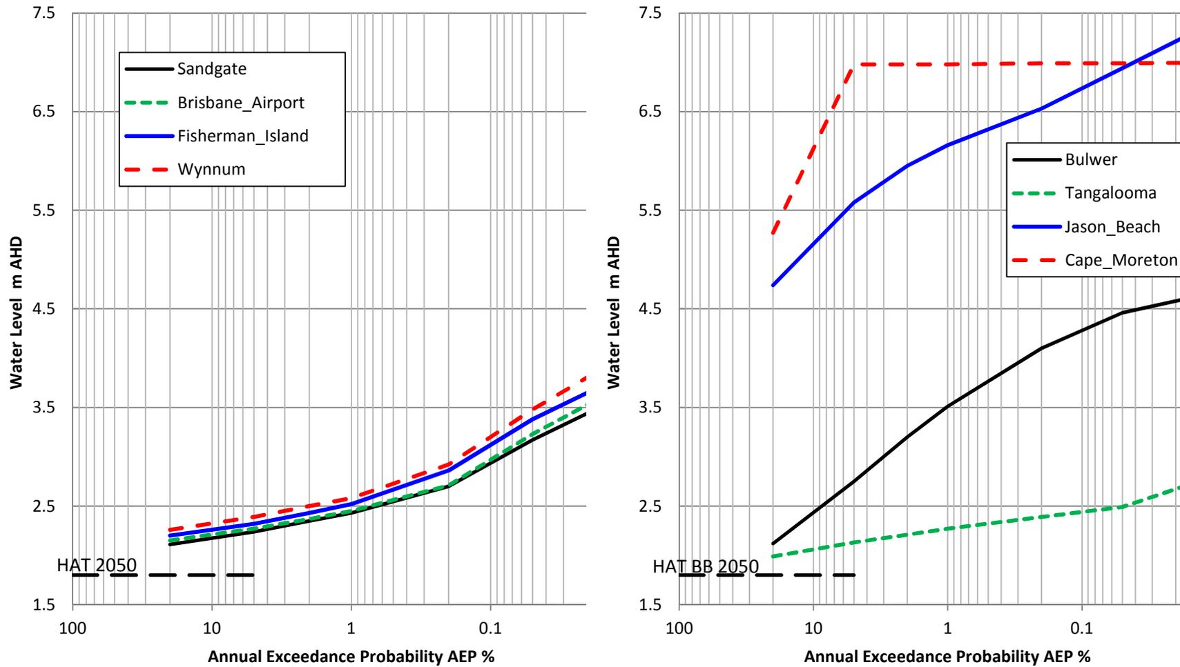
Figure 7-5 Combined 2050 climate breaking wave runup estimates at selected sites<sup>23</sup>
