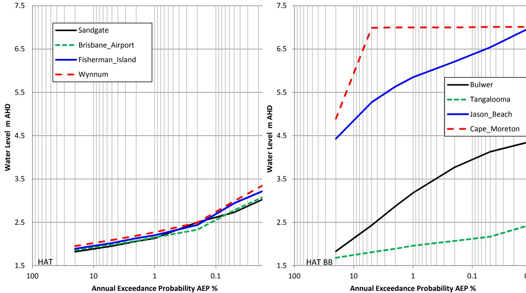
Figure 6-4 Combined climate breaking wave runup estimates at selected sites<sup>20</sup>
