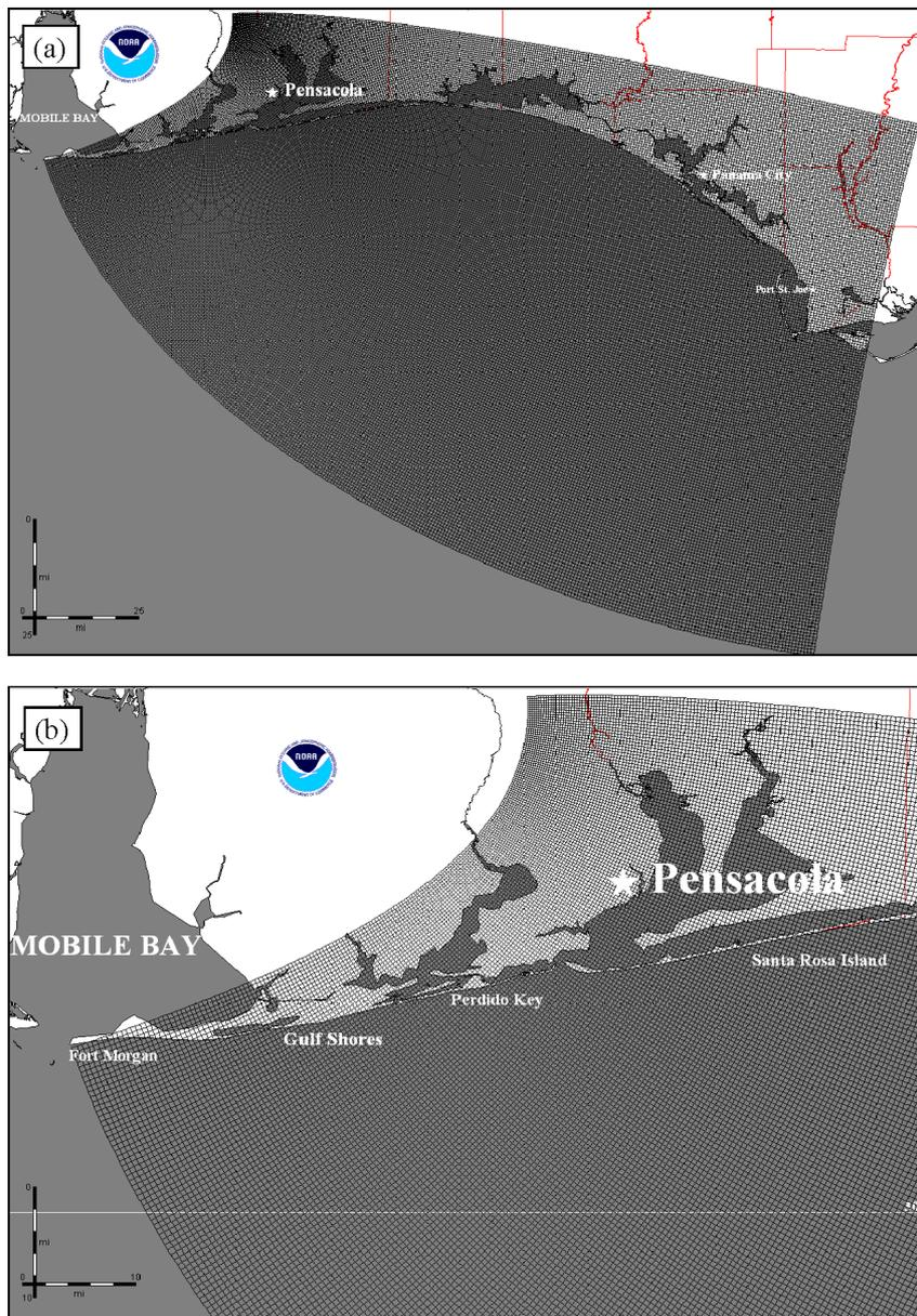
**Figure 2.** Finite difference storm surge model grid: (a) orthogonal curvilinear grid domain and (b) grid detail around Pensacola Bay. Figures provided by the US National Oceanic and Atmospheric Administration National Weather Service.
