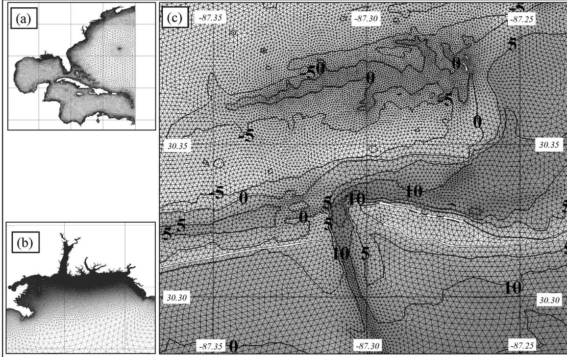
**Figure 3.** Finite element storm surge model grid: (a) unstructured grid domain, (b) high resolution grid in project region, and (c) model grid and bathymetry for the inlet to Pensacola Bay (m NAVD 88). Figure provided by the US National Oceanic and Atmospheric Administration National Ocean Service.
