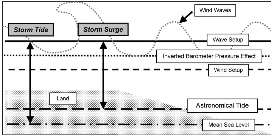
**Figure 1.** Contributions to the total water level during a severe storm surge event as it reaches land (gray shading). The individual effects vary significantly, depending on a variety of factors and this illustration cannot be construed as specific to any one case.
