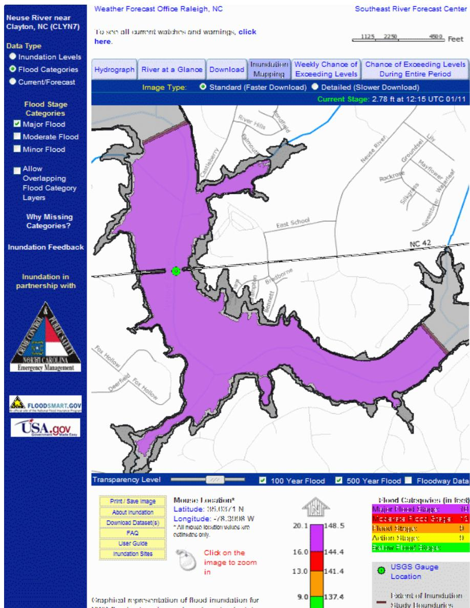
**Figure 15.** Inundation map for the Neuse River near Clayton, North Carolina, USA. (<http://newweb.erh.noaa.gov/ahps2/inundation/inundation.php?wfo=rah&gage=clyn7>)
