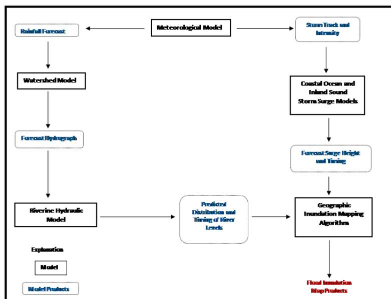
Figure 14. Suite of models required to simulate inundation from storm tides and upland flooding.
