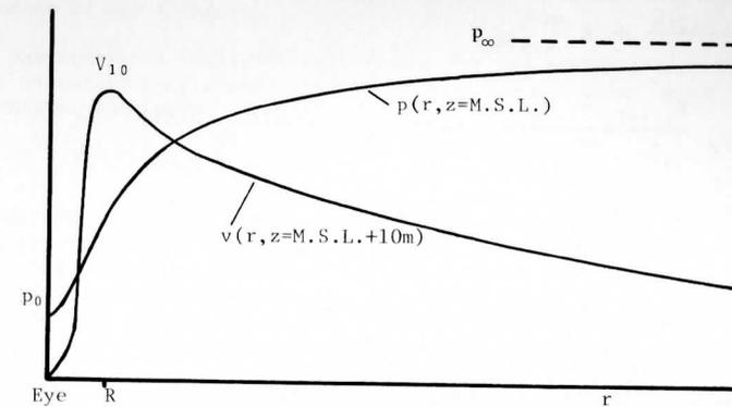
FIGURE 1. TYPICAL WIND VELOCITY AND PRESSURE PROFILES WITHIN A TROPICAL CYCLONE
