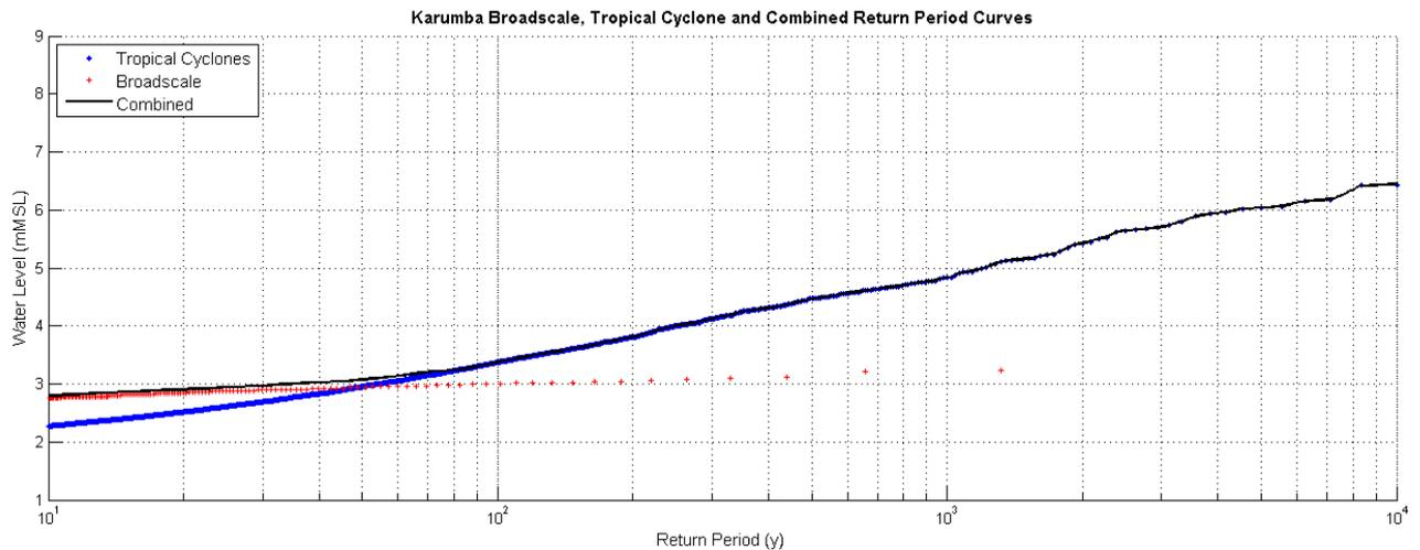
Figure 9 Broadscale (red), TC (blue) and statistically combined (black) tide plus surge Return Period curves for Karumba. Here broadscale events exceed TC level up to approximately 50 y. Note that combination (black) leads to estimated water levels that exceed either broadscale or TCs for levels with Return Periods ranging from 10 to 80 y
